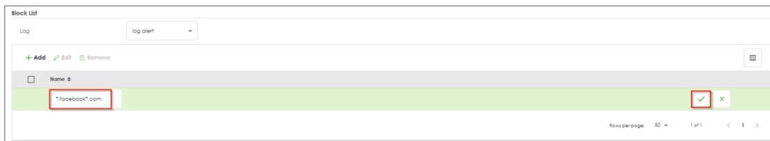
The screenshot shows the "Block list" configuration page. The "Log" dropdown is set to "log alert". Below the navigation buttons (+ Add, Edit, Remove), there is a table with one entry. The entry has a checkbox, the name "\*.facebook\*.com" (highlighted with a red box), and a status icon (a green checkmark in a box, also highlighted with a red box). The footer shows "Rows per page: 50" and "1 of 1".
