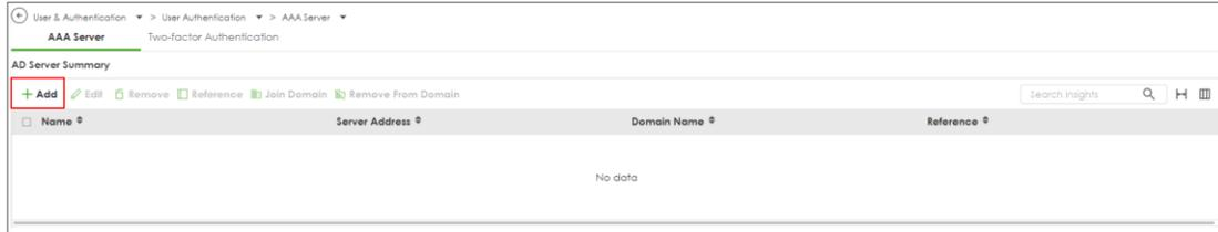
Enter the Server Address and port for Server settings. (10.214.48.XX:389 in this example). Enter the domain name and the credentials for logging into the AD server, and click Apply.
