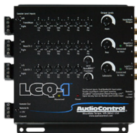
LCQ-1™ | SIX CHANNEL EQUALIZER AND LINE OUTPUT CONVERTER WITH ACCUBASS® AND SIGNAL SUMMING
