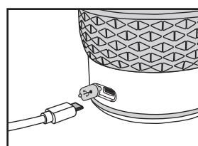
**Important: Do not use fast charging adapter. Use standard DC 5V 2A adapter.**
