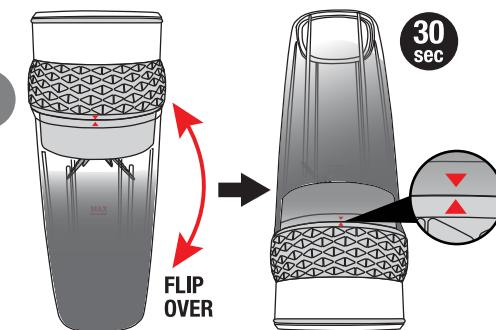
**• Flip the unit over and place it down on flat and leveled surface for blending.**
