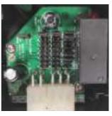
ON 10S LK4 is set; LK3 is set to S; LK1 is set to 1; OFF 10S LK6 is set; LK5 is set to S; LK2 is set to 1.
