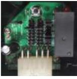
ON 30S OFF 30S LK4 is set; LK6 is set; LK3 is set to S; LK5 is set to S; LK1 is set to 3; LK2 is set to 3.
