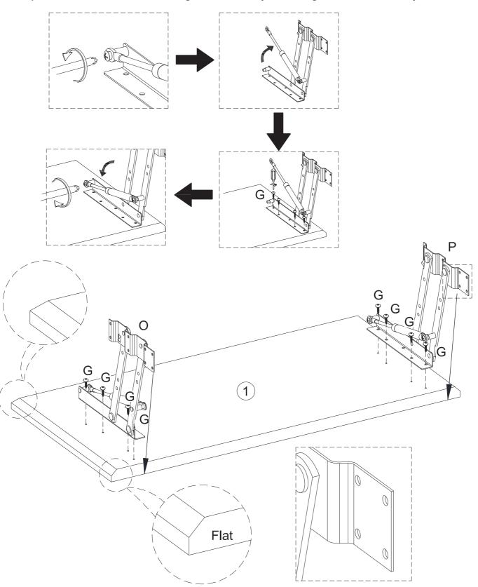
The side of part O/P with 4 holes and the flat side of panel  ${\mathbin{\textcircled{1}}}$  should be on the same side.
