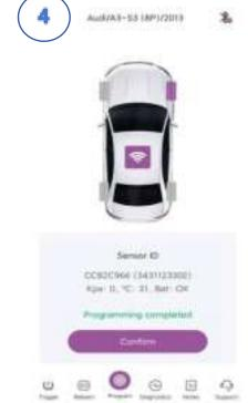
Once successfully programmed, the tool will display the sensor's ID, pressure,temperature and battery status.
