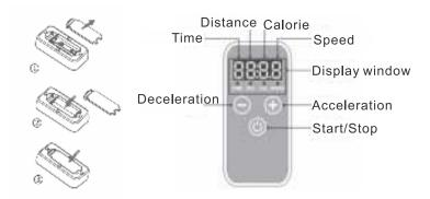
The following functions are displayed in the remote control window: time, speed, distance, and calorie data are displayed in the window in turn.
