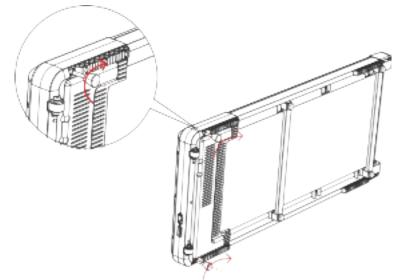
2.Foot pad adjustment: If the ground is uneven or the treadmill is shaking, please adjust the four adjustable foot pads at the bottom of the treadmill to appropriate positions, the foot pads must fit the ground. (As shown below)
