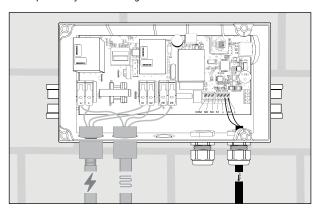
Figure 2.4 Temperature sensor wiring
