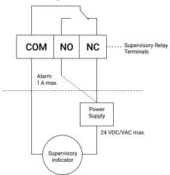
Figure 2.5 Supervisory relay wiring
