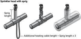
Figure 1.2 Installing XL-Trace on the sprinklers
