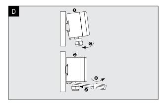
Figure 2.1 Mounting procedures for the 465 controller
