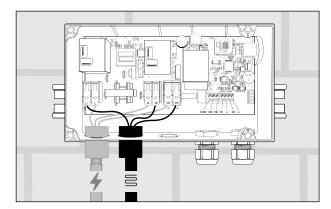
Figure 2.3 Heating cable connection
