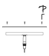
Install the glass lampshade on the lamp panel with screws.
