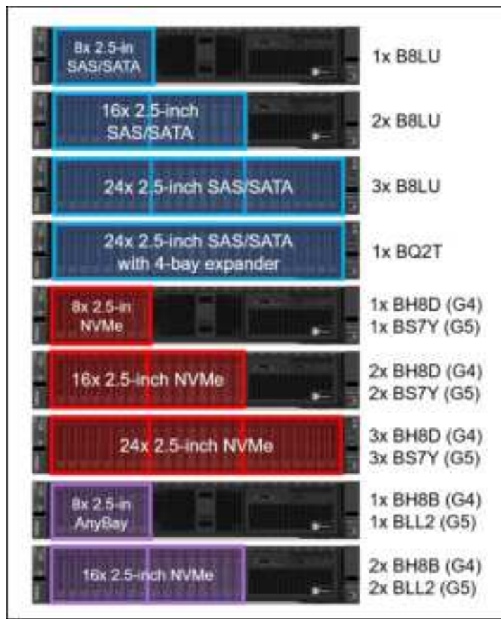
Figure 10. SR650 V3 front drive bay configurations - 2.5-inch drive bays, all the same drive type
