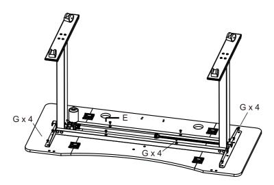
X 1 X 1 Install K -AC Adapter,B -Controller on the desktop. Controller 4mm Allen Key X 6 Screws M6x12 X 1 AC Adapter X4 Screws M4×12 F X 1 Type-C X 1 3mm Allen Key
