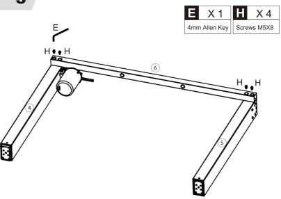
Install the another ⑥ -Support Beam on the other side in the same way as in step 3.
