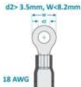
18 AWG wire with ring terminal for DC power supply
