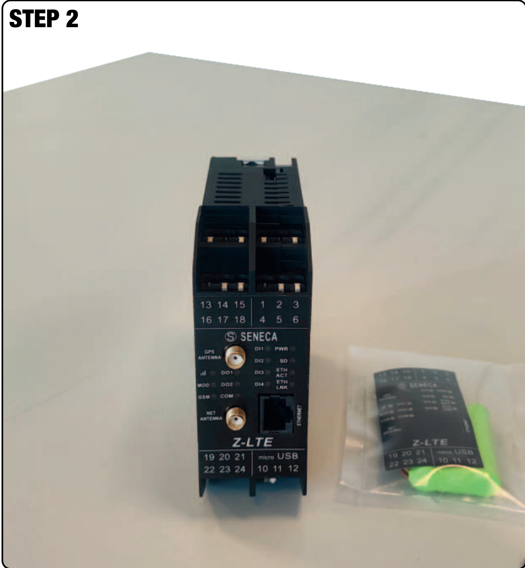
With the help of a screwdriver, remove the product terminals and DIN rail mounting hooks.
