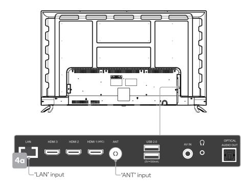
Following these options, the **Auto Tuning** screen will appear. Ensure you have an antenna cable connected to the 'ANT' input port at the back of the TV **(4a)**.
