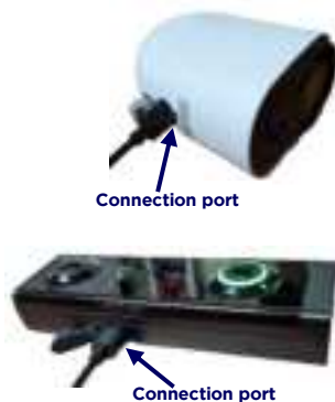
Figure 4: Connecting to Outdoor Camera and Wireless Doorbell
