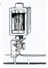
Connect the cold lead wires to power supply wires using approved wire connectors. Attach the braid pigtail to ground using the ring tongue terminal provided. Install the box cover.
