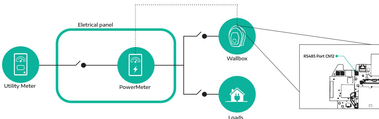
2. For the three-phase or single-phase electrical connection, refer to the dedicated meter installation manual included in the Power Meter package.
