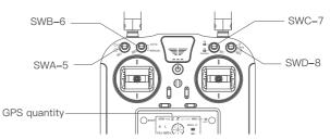
Toggle the switch upwards, and the helicopter will record the current coordinates, then fly horizontally figure 8 based on these coordinates.
