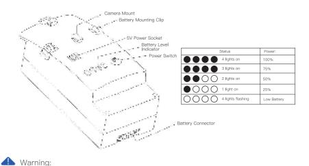
After use, please turn off the battery as prolonged power-on time may shorten the battery lifespan. After flying, remove the battery from the cabin to prevent damage due to over-discharge.
