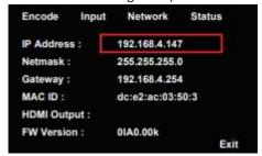
**3.2** Open the browser and input the IP address, e.g. 192.168.4.147, to access the login interface.
