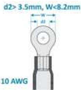
10 AWG wire with ring terminal for DC power supply
