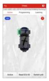
Tap Read ECU ID. Connect the tool to the vehicle's DLC port and tap OK to start reading the sensor IDs and positions for viewing.
