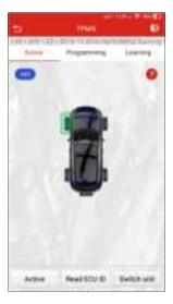
For universal sensors, place the TPMS antenna of the tool alongside the valve stem, point toward the sensor location, and tap **Activate** on the screen.
