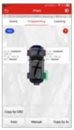
\*Note: If Auto Create is selected, the TPMS Relearn operation needs to be performed after programming all required LAUNCH-specific sensor.
