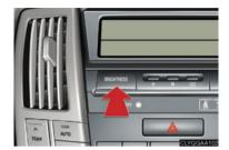
To adjust the brightness of the multi-display light, press the button repeatedly until the desired brightness is obtained.
