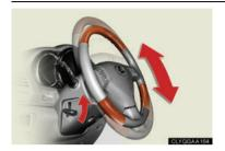
To adjust the steering wheel, pull the lever up while holding the steering wheel, tilt the steering wheel to the desired angle, and release the lever.
