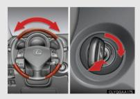
Turn the engine switch while lightly moving the steering wheel from left to light.
