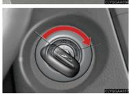
2 Turn the engine switch to the START position.
