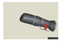
The fog lights can be used only when the headlights (low beam) are on.
