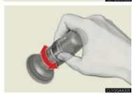
To spray washer fluid, pull the lever. The wipers will operate automatically.
