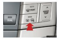
To defog the rear window and the outside rear view mirrors, press the button.
