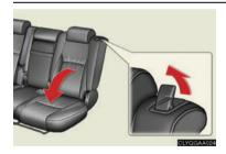
Pull the lever and fold the seatback down until it locks.
