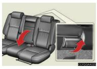
Pull the lever behind the center seatback and fold the seatback down.
