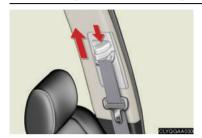
To raise: push the anchor upward.
