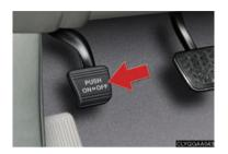
To set the parking brake: firmly depress the parking brake pedal.
