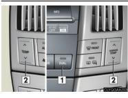
In DUAL mode, driver and passenger side temperature settings can be adjusted separately.
