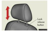
To raise: push the head restraint upward.
