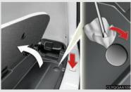
2 Open the right side auxiliary box and remove the cover of the spare tire clamp bolt.
