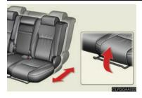
With the lever raised, slide the seat forward or backward.
