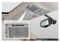
The HomeLink<sup>®</sup> compatible transceiver in your vehicle has 3 buttons which can be programmed to operate 3 different devices.
