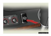
The headlight cleaner can be used only when the engine switch is in the ON position and the headlights are on.
