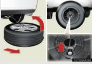
4 Pull out the spare tire and remove the holding bracket.
