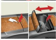
To adjust the position of the front console box, open the cup holder lid and slide the console box while lifting the lever.
