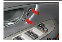
While holding down the SET button, press and hold memory button 1 or 2 until you hear a beep.
