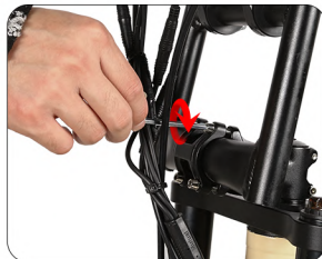
Tighten 4 screws to fix the handlebar
