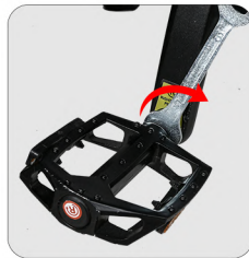
Tighten the right pedal "R" clockwise
