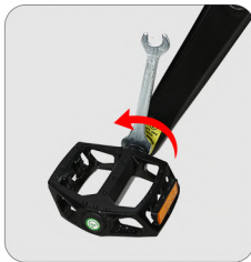
Tighten the left pedal "L" counter clockwise
