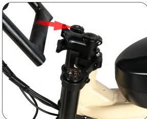
Install the handlebar to adjust the direction
