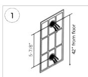
Install 1/2'' hot  $\theta$  cold supplies at 42" height from the finished floor and 5-7/8" apart on center. Use the included NPT to G thread adapters and make sure the end of the adapter does not protrude from the finished wall.
