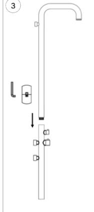
Assemble the fixture by inserting the upper part into the lower part. Align the indicator on the back of the fixture and tighten the set screw.
