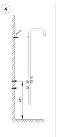
Hold the assembled fixture in place and mark the position of the upper bracket. Then, install the upper bracket.
