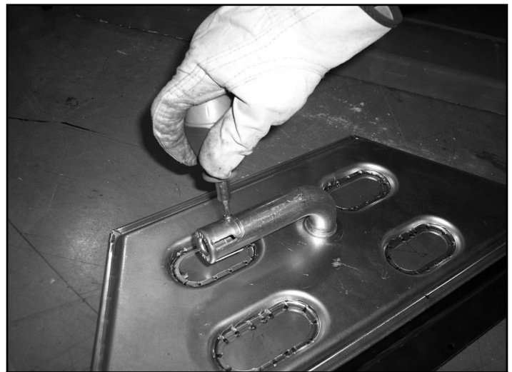
Figure 12.19 Adjust Air Shutter
