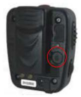
Ensure your BluSkye® Speaker Microphone (SM) is powered off. Press the power button for 6 seconds. The SM will beep twice at 3 seconds, and twice again at 6 seconds. The LED will begin to alternate between blue and red.
