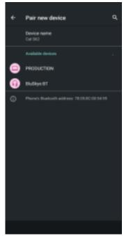
For devices without NFC, navigate to Settings > Connected Devices > Pair New Device. Select BluSkye BT.
