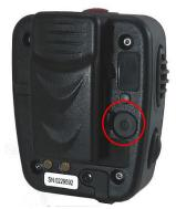
1. Ensure your BluSkye® Speaker Microphone (SM) is powered off. Press the power button for 6 seconds. The SM will beep twice at 3 seconds, and twice again at 6 seconds. The LED will begin to alternate between blue and red.
