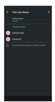
4. For devices without NFC, navigate to Settings > Connected Devices > Pair New Device. Select BluSkye BT.
