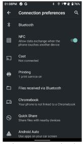
2. For devices equipped with NFC, navigate to Settings > Connected **Devices > Connection Preferences** and toggle NFC on. For devices
