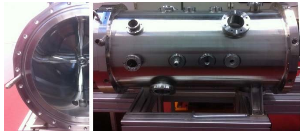
Figure 2: The 325 MHz high-field cavity before the copper plating.
