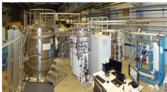
Figure 1: The HeSu plant. From right to left: purifier cold box and LHe storage
