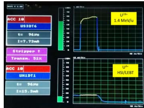
Fig. 2: Beam transformer measurement after careful optimization of a VARIS-uranium beam.
