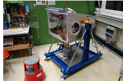
Figure 2: The testing chamber for motor drive units.
