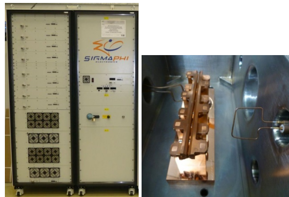
Figure 2: Amplifier (left) and RFQ test cavity structure.
