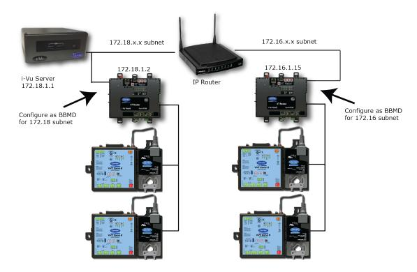
If your system has multiple routers that reside on different IP subnets, you must set up one router on each IP subnet as a BACnet/IP Broadcast Management Device (BBMD).
