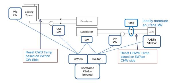
Even though the controller works with a variety of chilled water system components, it must be used with parallel chiller systems and operates best with variable speed pumps and variable speed fans.
