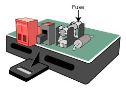
**6** Use the fuse puller to snap the new fuse into the fuse holder.
