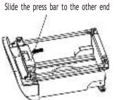
Install the trash bag by hanging the four holes of the trash bag to the pins of the waste collecting drawer.
