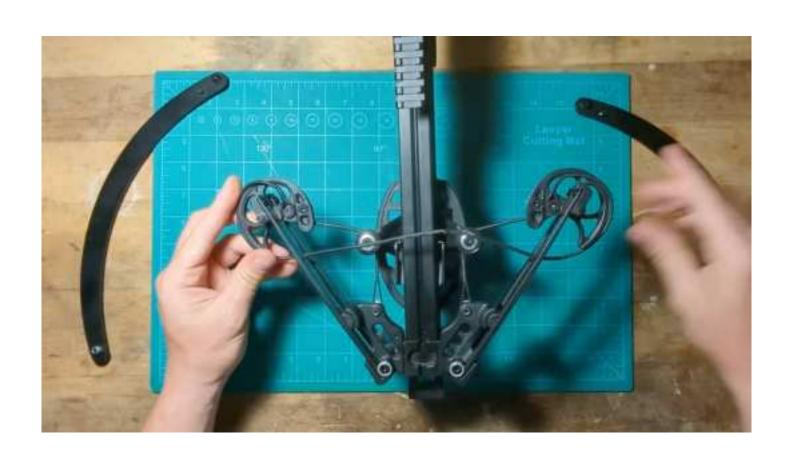
7. Insert the string along the grooves in the cams.
