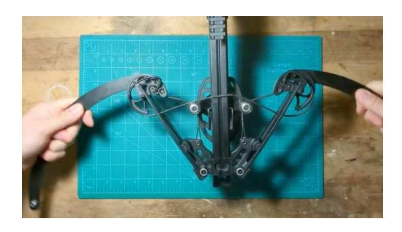
6. Insert the press bars in the cam openings and fasten them.
