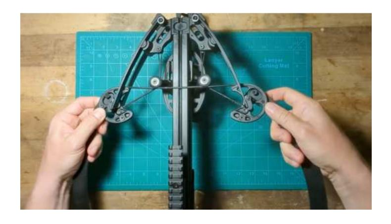
3. Turn the crossbow over. Unscrew the bolts that secure the cables to the crossbow body.
