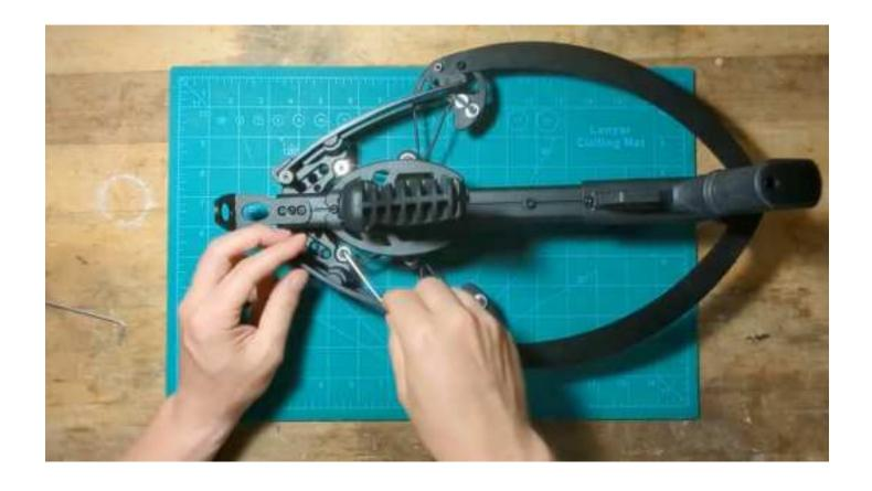
5. After replacing the cables for new ones, attach them to the crossbow body and cams.
