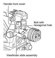
3 Attach the handle front cover with the bottom edge up.
