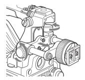
2 Using a 2.5 mm diameter hexagonal wrench, detach the viewfinder slide assembly and handle front cover.
