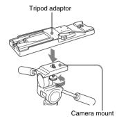
2 Mount the camcorder on the tripod adaptor.
