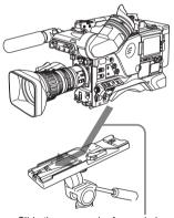
Slide the camcorder forward along the groove in the adaptor until it clicks.
