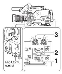
1 To adjust the signal input to the AUDIO IN CH1 or CH2 connector, set the AUDIO IN CH-1 or CH-2 switch to REAR.
