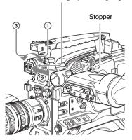
2 Couple the viewfinder connector to the VF connector.
