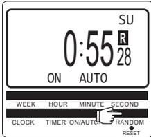
When starting the random mode, the timer will turn on and off randomly with a 2-32 minute variation based on the on and off schedule you set. The RANDOM function can only work when the timer setting is finished, and the time is in auto mode. Press "RANDOM" again to exit the Random mode.
