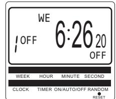
**NOTE:** Repeat press "TIMER" to enter different ON/OFF programs. The timer allows for a maximum of 20 ON/OFF settings to be programmed.
