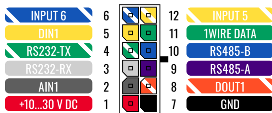
FMB125 2x6 socket pinout
