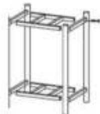
**Note:** Be sure to tighten the screws half way first. Only when the shelves are properly straight, tighten all screws.
