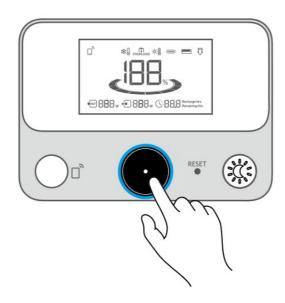
Press the main power button for 3 seconds to turn your power station on or off.
