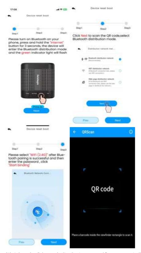
(3) Select the "Bluetooth distribution network" to automatically search for Bluetooth signals and pairing. After successful pairing, jump to WiFi interface. Please select 2.4Ghz WiFi and enter the password.
