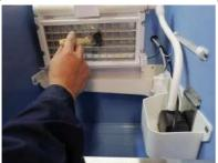
3.4 Use a cross screwdriver to remove the fixing screw on the ice shower pipe, and then remove the left and right plug and the shower pipe at one time. Then clean the pipe inside and outside of the shower pipe with a brush.
