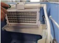
3.3 Wash the ice lattice surface with a soft brush or sponge dipped in vinegar or scale remover to clean up the scale.
