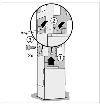
3. Hook in the retaining clip and screw tight.
