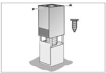
**5.** Insert both lower parts of the flue and push together.
