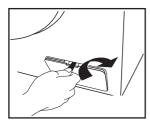
Open the filter cover with tools such as coins according to the direction of the graphic;
