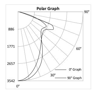
Note: All published photometric testing performed to IES LM-79-08 standards. Fixture photometry was completed on a single representative fixture. Foot candle levels are noted inside graph.
