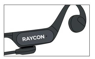
Plug into a Power Source: Plug the USB end of the charging cable into a USB power source, such as a computer, USB wall adapter, or power bank. Ensure the power source is reliable and functional.
