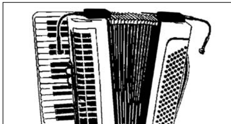
Fig. 6: Miking up an accordion with two C 516 MLs.
