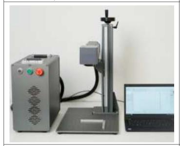
5.Press "light" to ensure it'll mark on the test material. Click "mark", and the laser is in continuous marking state
