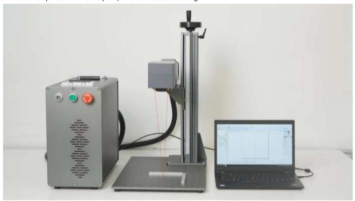
Note: Before the machine is out of the factory, we have done red light correction. At the position where the three red light spots are focused, the laser emits the strongest light. However, due to transportation reasons, the focus point of the red lights you received may shift, and the focus point is not the best focal length. Please refer to FAQ 2 at the back of this manual for debugging.
