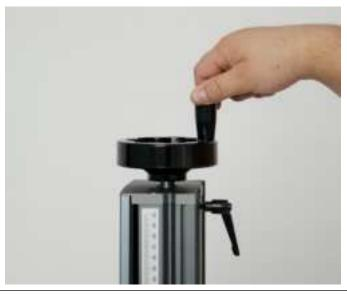
8. Manually adjust the relative position of the red light dots to make them overlap. And tighten the screws
