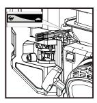
5. Pull the recoil starter until engine compression has become difficult to pull. Let the recoil return to the home position, then pull quickly to start the engine. Repeat steps as needed. Fully open the choke.
