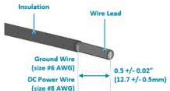
6-AWG green-and-yellow wire for grounding 8-AWG DC power wire
