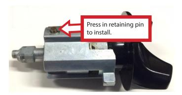
**STEP 2:** Insert lock into column. Ensure that cylinder is fully seated and aligned in interlocking washer before turning key to the off position. This will enable the lock retaining pin to extend into cylinder housing.
