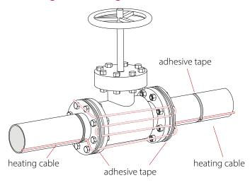
• In areas with large pipe diameters, heating cables must be laid in a loop.
