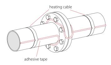
When laying a heating cable around a flange connection, it must be ensured that the heating cable is laid once around the pipe directly in front of the flange connection. More power must be applied to the pipe at this point due to higher thermal expansion.
