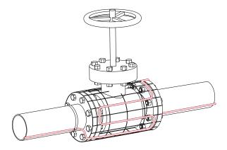
• Fasten the heating cable onto the braiding
