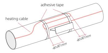
• In areas of pipe supports, heating cables must be laid in a looped manner in order to be able to provide sufficient power at this point.
