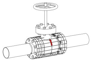
Fasten the braiding onto the fitting
