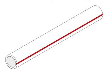
Normally the heating cable is laid streched out along the pipe. Lay heating cables in a spiral pattern only if the projects planning explicity calls for it.
