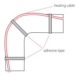
• When laying a heating cable around a pipe bend, the heating cable must be laid on the outside of the pipe bend. If it is laid on the inside, the flow medium may be deposited in the pipe due to the lower heat input to the pipe.
