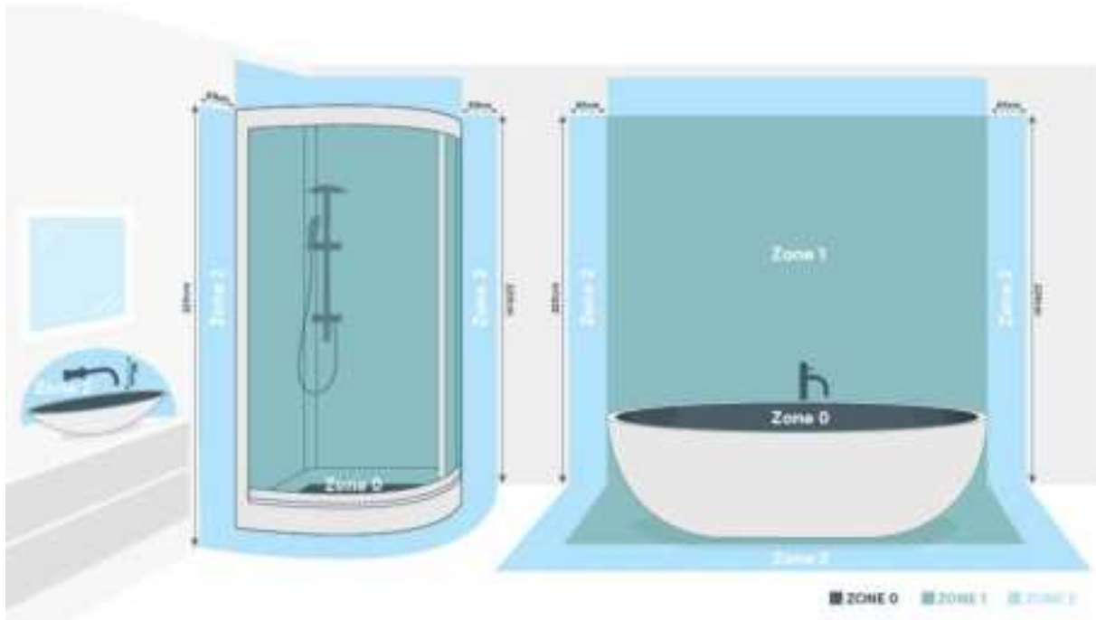
Figure 1 | Bathroom installation zones
