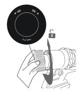
1 Turn the HEPA filter counter -clockwise to remove
